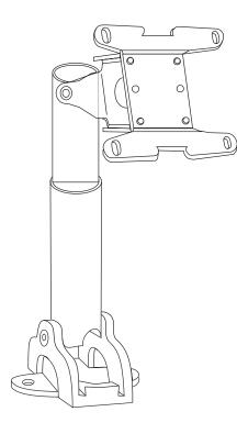
Typical Pedestal Type Mount with Swivel Bracket
