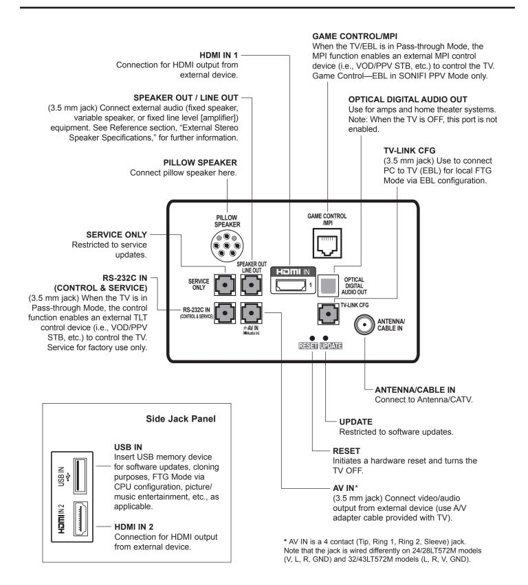
The SPEAKER OUT / LINE OUT 3.5 mm stereo jack on the LT572M rear panel provides stereo speaker signal outputs (fixed speaker, variable speaker, or fixed line level [amplifier]) for external audio equipment. Set Installer Menu item 097 AUDIO OUTPUT as required in accordance with external audio equipment connected to the TV. Also, refer to the following diagram for pinout details.
