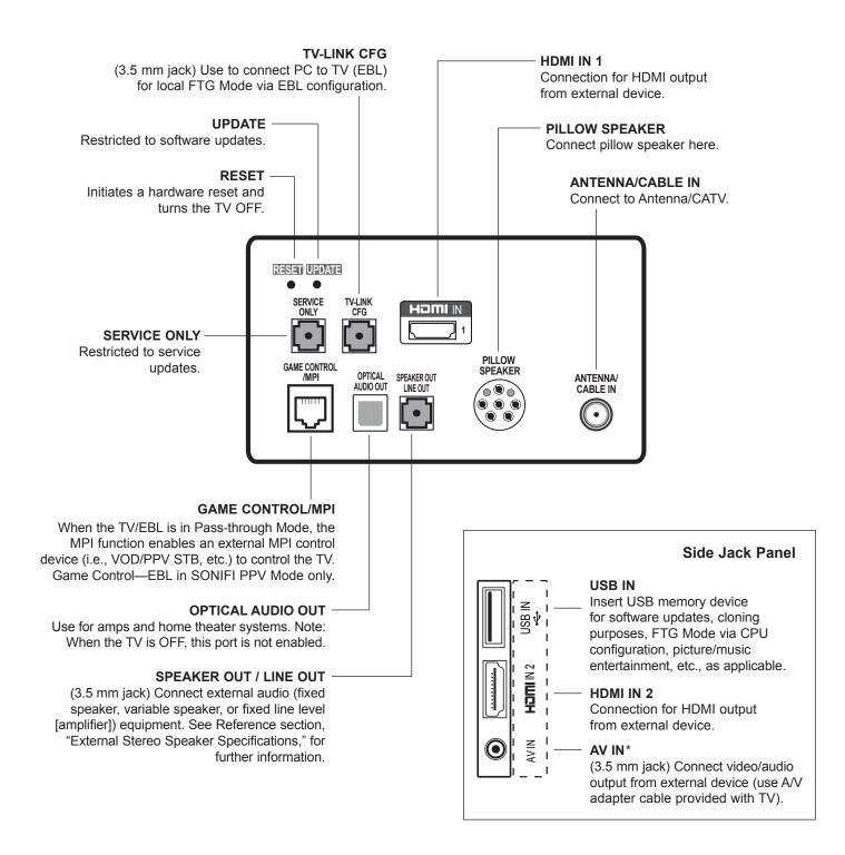
\* AV IN is a 4 contact (Tip, Ring 1, Ring 2, Sleeve) jack. Note that the jack is wired differently on 24/28LT572M models (V, L, R, GND) and 32/43LT572M models (L, R, V, GND).
